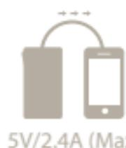
Plug in your device to the Power Bank's output port via a USB charging cable.
